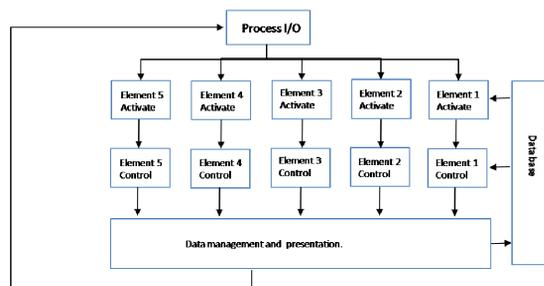
Figure 5: Vacuum control system block diagram.
