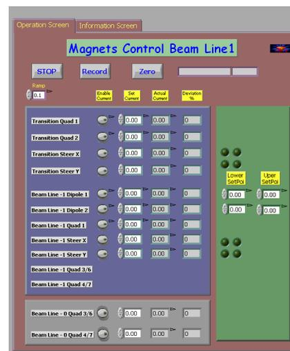
Figure 1: Beam lines magnets control system HMI.
