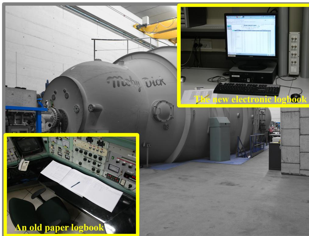
Figure 4: The external tank of the LNL 15 MV Tandem electrostatic accelerator with photos of an old paper logbook and of the new system.
