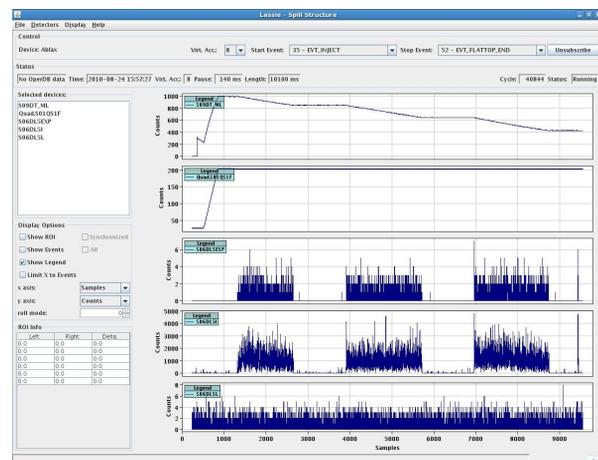
Figure 1: The LASSIE spill structure tool for analysis of synchrotron signals (from top to bottom: current transformer, quadrupole ramp and beam loss monitors).
