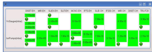
Figure 5: Labels from cabling are used to group in grids the experimental equipment pressures.
