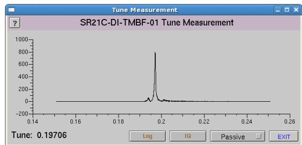
Figure 10: Online tune measurement (horizontal plane). The raw IQ data from FPGA can also available as Epics waveforms.
