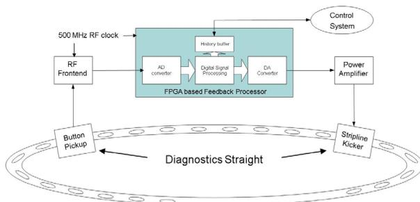
Figure 1: Block diagram of the Diamond TMBF system.
