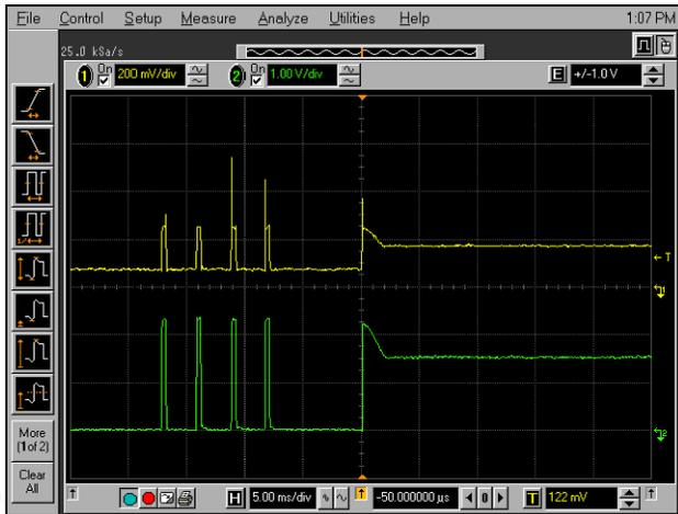
Figure 2: The waveform of forward and reflect power.
