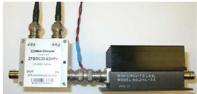
Figure 5: The picture of amplifier and directional coupler.
