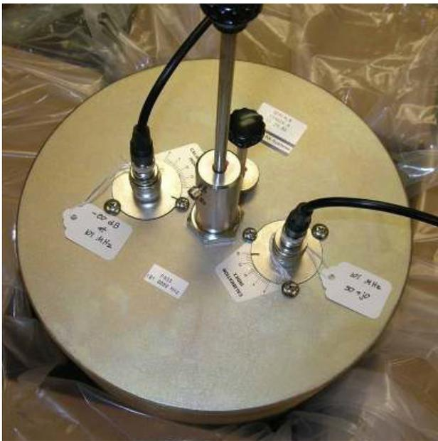
Figure 4: The picture of resonant cavity.
