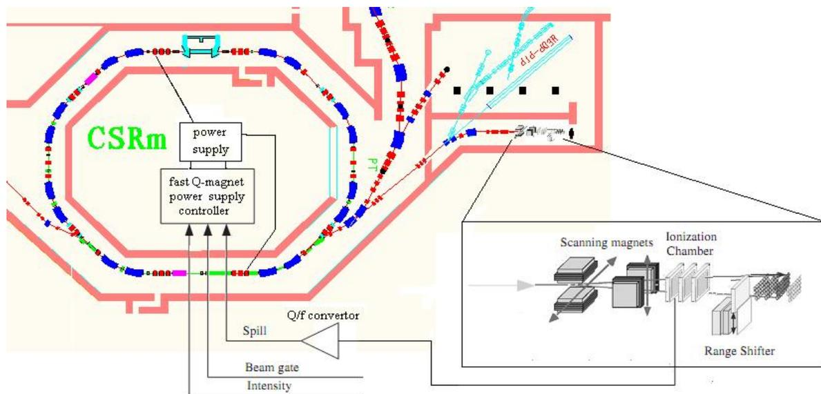
Figure 2: Block diagram of the spill feedback system.
