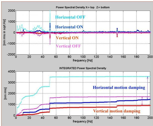
Figure 5: Beam motion averaged over 224 BPMs.
