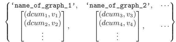
Figure 3: Final structure of “plotdict” object after data combining.  $dcum_1$  is the position of BLM<sub>1</sub>, and  $v_1$  the signal of BLM<sub>1</sub> at the plotting time. See Fig. 5 for the corresponding graph.
