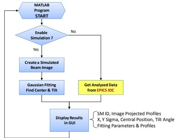
Figure 5: Flow chart of Matlab display GUI.
