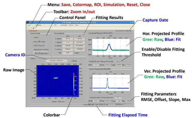
Figure 4: Layout of the Matlab display GUI.
