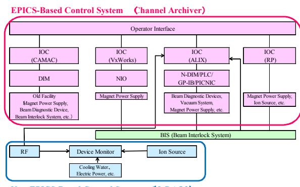
Figure 1: Schematic of RIBF Control System.
