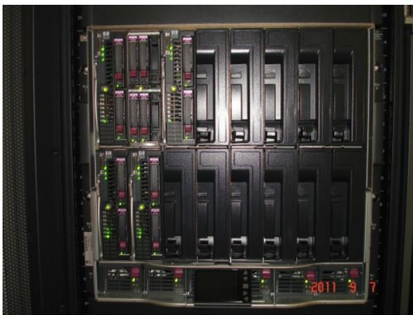
Figure 4: The blade enclosure.
