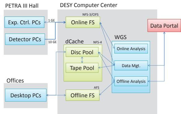
Figure 5: Main data and control flow paths.
