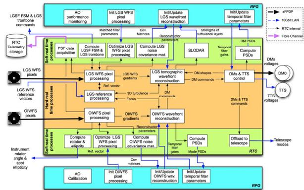
Figure 2: Top-level RTC control block diagram for the LGS AO operation mode. The RTC works in synchronization with the Reconstructor Parameter Generator (RPG – blue boxes). The RTC processes are split into two categories: the hard real time processes (orange) and the background and optimization processes (green). Finally, but not least, the RTC design should be modular to allow the system to be modified or upgraded for the next generation of AO systems.
