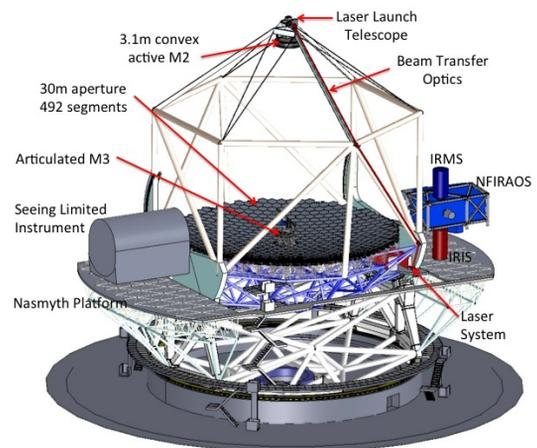
Figure 1: TMT telescope overview and first light instrumentation.
