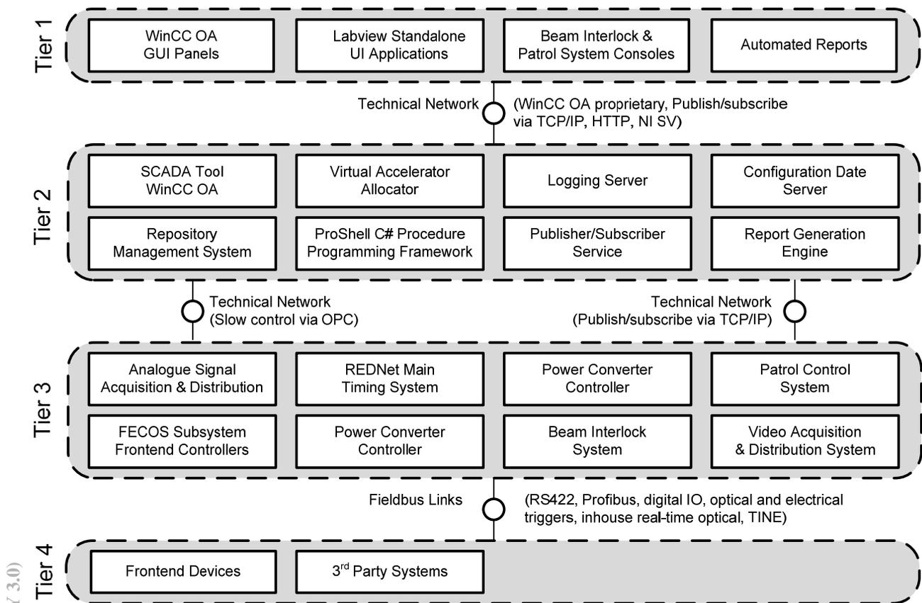
Figure 2: 4-tier accelerator control system architecture. Tier 4 comprises low-level front-end devices or third party control systems that must be integrated via a proxy front-end controller at tier 3. A single physical technical network permits communication among tiers in a secured network environment. Applications at tier 1 and 2 are virtualized.
