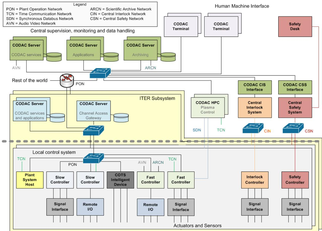
Figure 1: Physical architecture of ITER control system.
