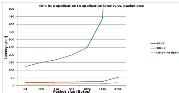
Figure 3. Measured latency 1GbE, 10GbE and RMN.
