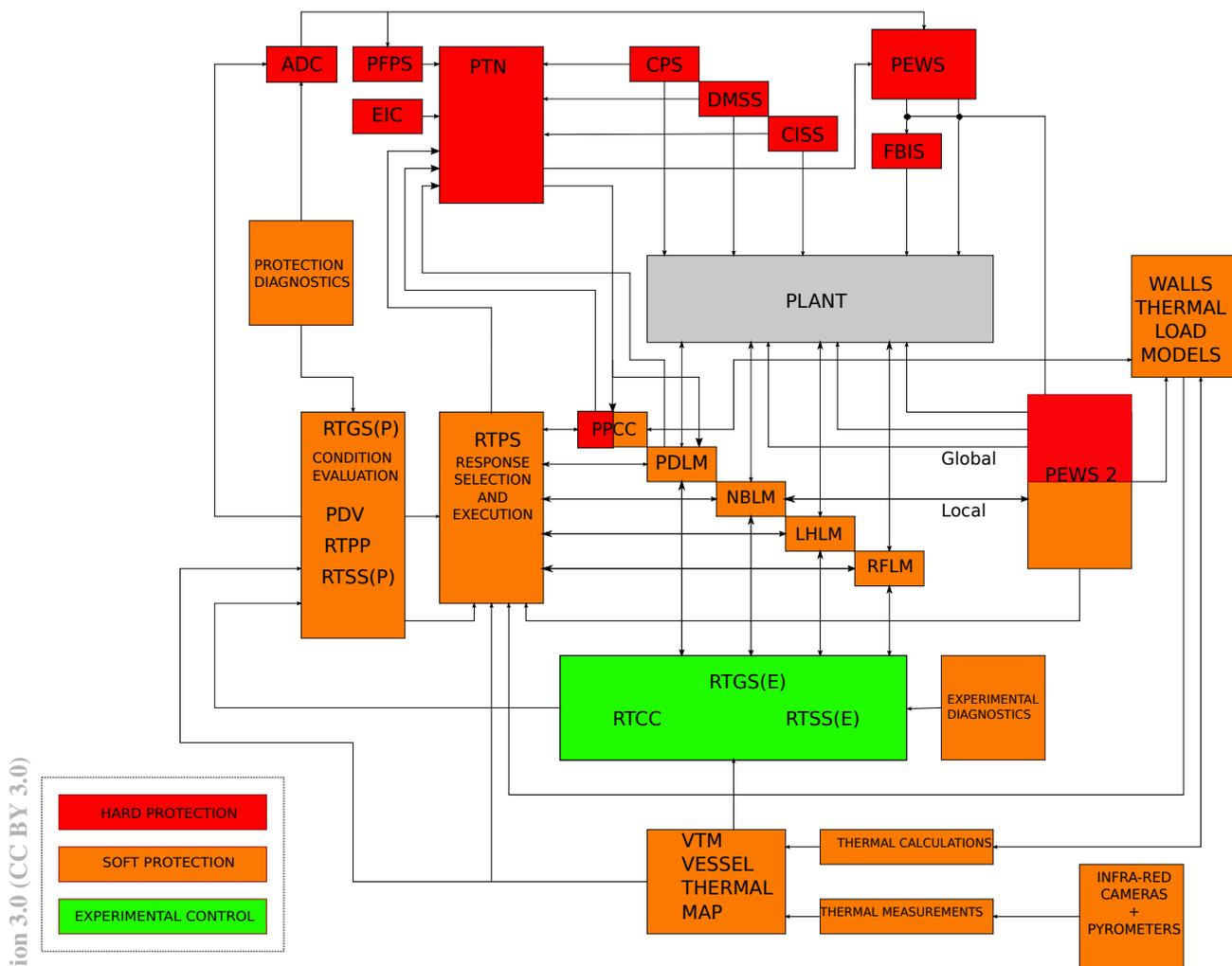
Figure 1: JET protection of the ITER-like wall system architecture. The experimental real-time control links to the density and heating local managers (PDLM, NBLM, RFLM and LHLM) is expanded to allow protection overrides from the new RTPS system which receives alarms from VTM, WALLS and also from the real-time plasma protection (RTPP) and real-time central controller (RTCC) systems. The original higher level protection systems of CISS, PTN and PEWS are retained.
