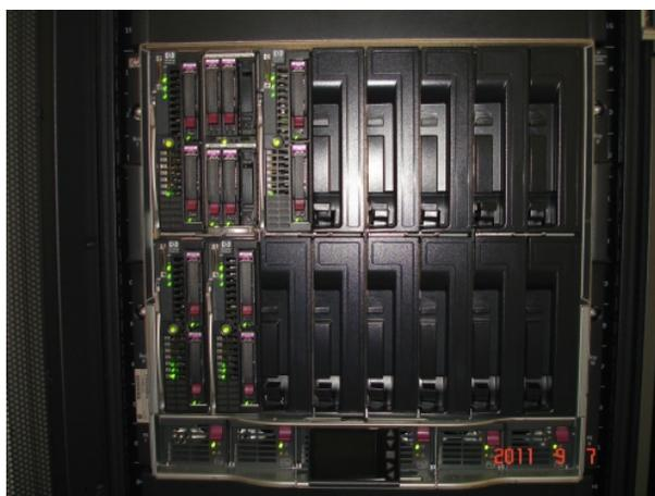
Figure 4: The blade enclosure.
