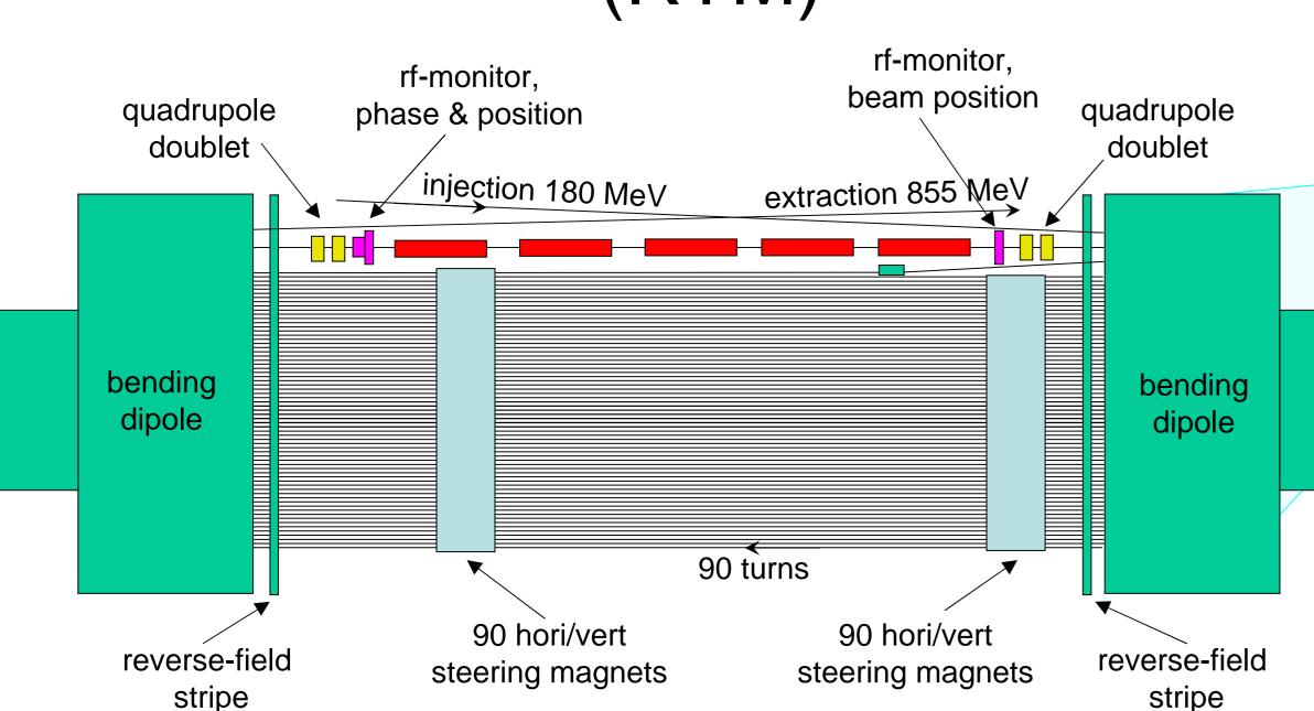
The 3rd RTM stage with an output energy of 855 MeV is in operation since 1990 and serves now as injector for the HDSM.
