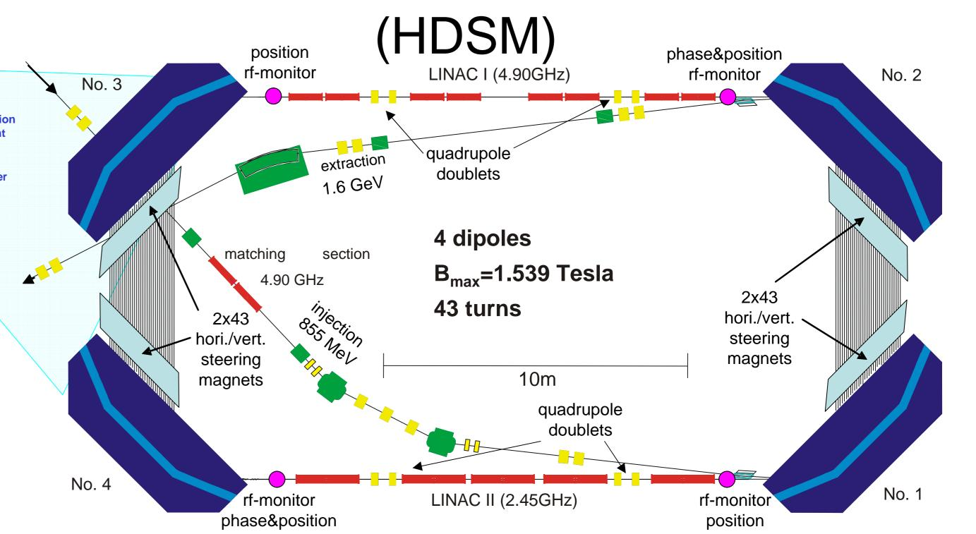
The 4th stage, boosting the energy from 0.855 GeV to 1.6 GeV, was built in parallel to regular operation of the first 3 RTMs. Its commissioning started in Dec 2006 and since Feb 2007 it is in routine operation for nuclear physics experiments.
