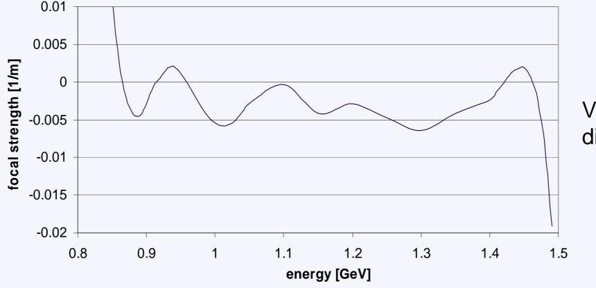
Vertical focal strength of the first dipole against beam energy.
