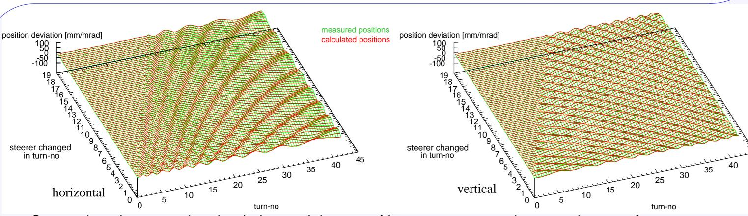
Comparison between the simulation and the actual beam responses due to a change of one steerer kick at a time in the first 19 turns. The right axis denotes the turn number in the HDSM, the upright axis the beam position variations due to a change of one steerer, whose position (in turn-no) is noted at the left axis (there are 4 steerers in each turn). The green lines show the measured beam position deviations, the red ones the deviations calculated by the adapted HDSM simulation.
