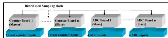
Figure 1: Multi-board data acquisition architecture.
