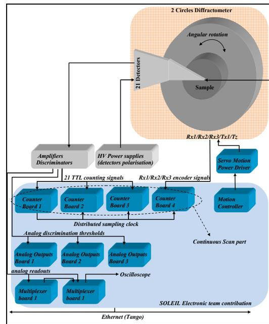
Figure 5: 2 Circle diffractometer architecture overview.
