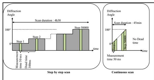
Figure 7: Timing comparison between step by step and continuous scan.
