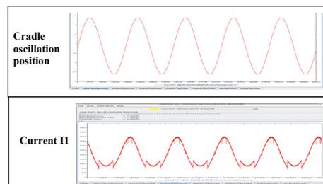
Figure 9: Acquisition buffer of oscillating cradle on counter board and current I1 on ADC board.
