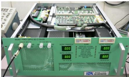
Figure 1: Front and top view of 2-channel type magnet power supply. The “i-DIO” is inserted from the rear panel.
