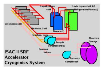
Figure 1: ISAC-II cryogenics system block diagram. Liquid Nitrogen delivery not shown.
