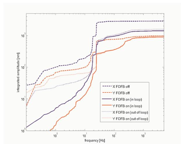
Figure 4: Integrated amplitude of positional noise for Feedback Off, Feedback On, in loop, and Feedback On, out of loop.
