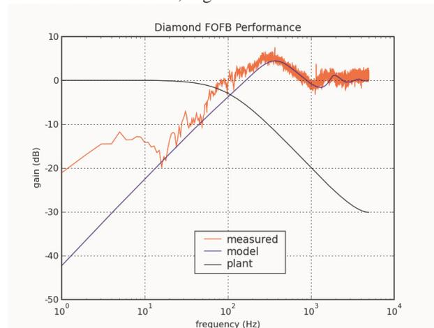
Figure 3: Theoretical and measured suppression in the vertical plane. Below 10 Hz is noise dominated in the measured data.
