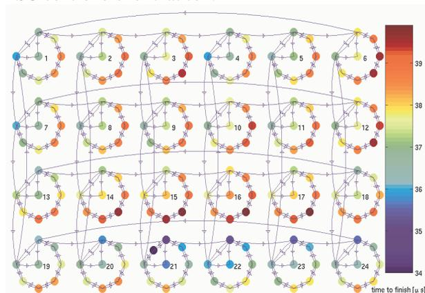
Figure 1: Communication network topology, with each circle being one cell consisting of seven eBPMs, and a computation node in the centre. The interconnection is as a 2D torus showing propagation delay between 34  $\mu\text{sec}$  and 40  $\mu\text{sec}$ .
