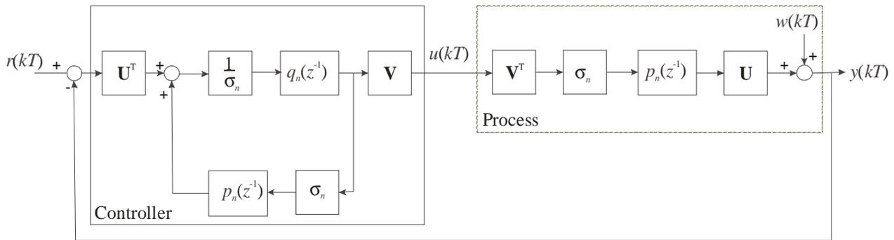
Figure 2: Feedback controller structure,  $r$  demanded orbit,  $u$  correctors,  $y$  measure orbit,  $p$  plant,  $q$  compensator for plant,  $\sigma$  singular values.
