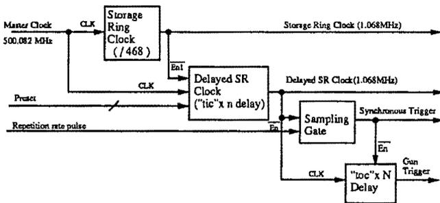
Fig. 4 Schematic Diagram of the Bucket Selector
