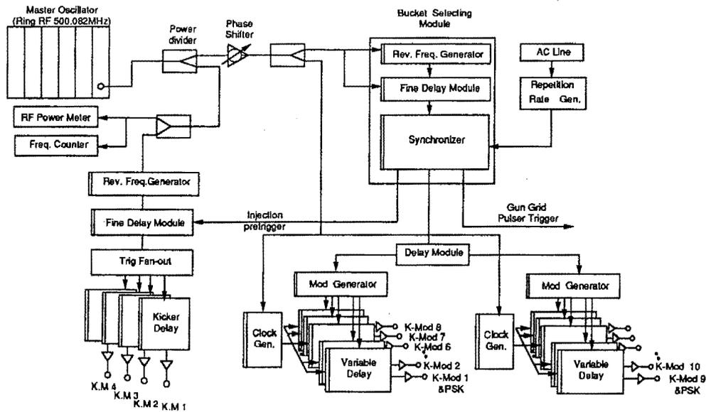
Fig. 3 Schematic Diagram of the PLS Timing System
