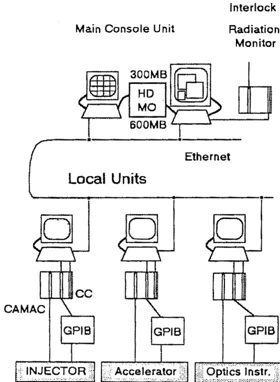
Figure 2. Schematic diagram of the hardware configuration.
