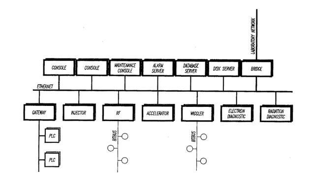
Fig. 2 - The hardware architecture of the control system
