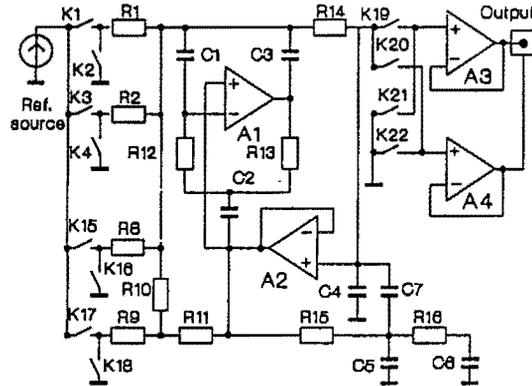
Fig.2. The analog section of multiphase PWM-DAC.
