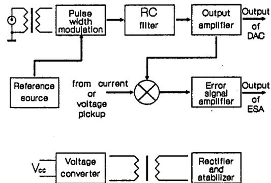
Fig.1. The analog section of PWM-DAC.
