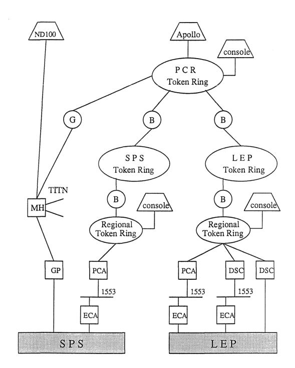
Figure 1 Logical schematic of the networks
