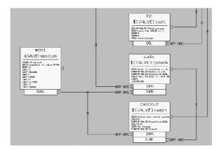
Visually Visual DCT resembles GDCT, users can create, move and link records. Fields can be modified, and any fields not using the default values are displayed. Data flow direction is indicated by an arrow. Records can be grouped together in a logical block, which allows a hierarchy of functions to be built, making the design easier to understand.
