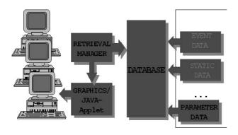
Fig1 Configuration of the Diagnostic System using DB
