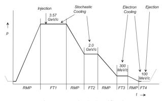
Figure1: AD Cycle Specification
