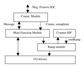
Fig 2. FDC software functional diagram
