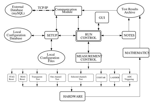
Figure 2. Measurement program architecture
