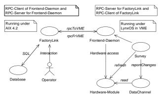
Figure 1: Client-server control system structure
