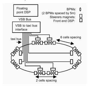
Figure 1: Layout of the global feedback system.
