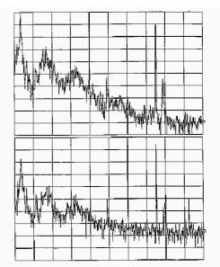
Figure 5: Spectrum of a dipole X ray beam position 25 m away from the source with feedback off and on (5dB/div, 200 Hz span).
