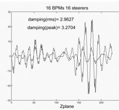
Figure 2: Example of static orbit correction obtained with our 16 BPMs/16 steerers system
