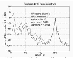
Figure 4: Spectrum of the beam position motion signal of a feedback BPM with feedback off and on
