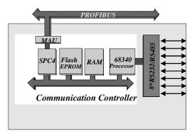
Figure 2: Block diagram of the serial gateway
