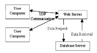
Figure 2: Data Transaction Scheme
