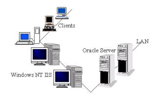
Figure 1: Client Server NW Scheme
