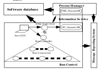
Figure 1: The RC in the context of Backend Components
