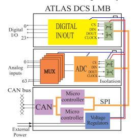
Figure 1 Block diagram of the LMB
