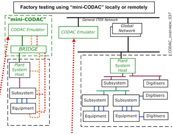
"Mini-CODAC" tests all CODAC interfaces and functionality at the factory, where the competence is. Either uploaded or remote from Cadarache.
