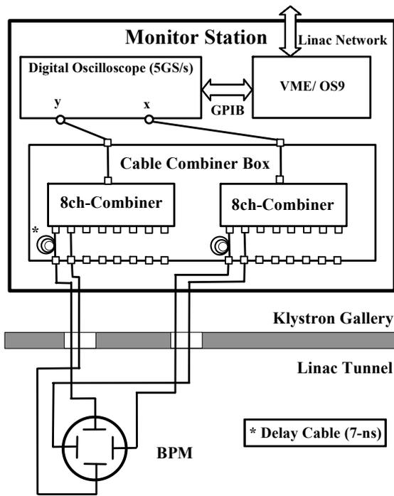
Figure 1: Schematic drawing of previous BPM DAQ system.
