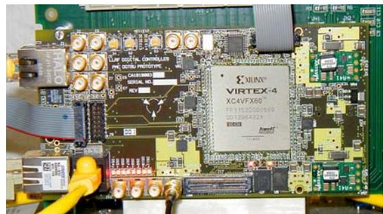
Figure 1: Custom design PMC module using ML310's 3.3V PCI slot to obtain power.
