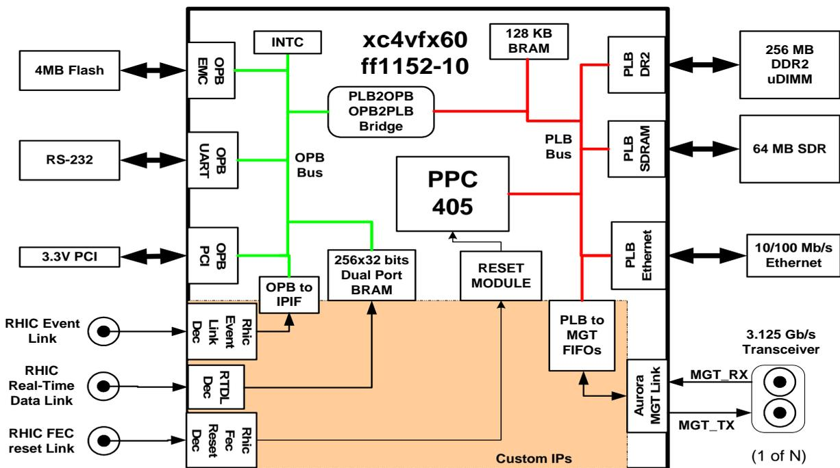
Figure 2: Block diagram of the embedded design.
