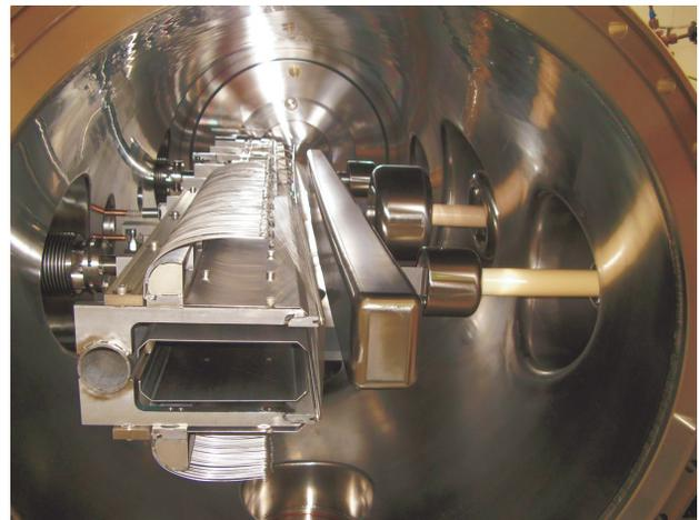
Figure 1: Electrostatic injection septum as seen from inside. Anode and cathode plate are being moved towards each other by the means of two parallel spindles per plate (plate holders extensions). Plates must be moved parallel and must never touch.
