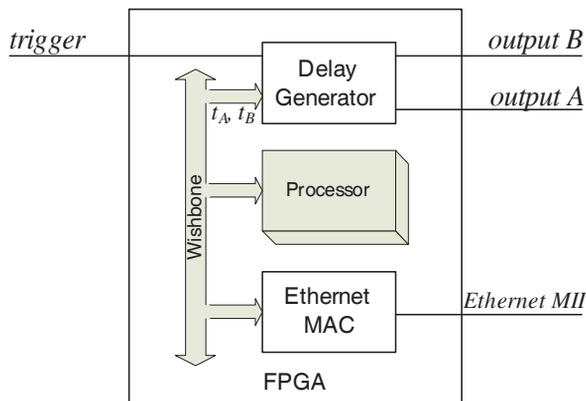
Figure 2: Block diagram of a delay generator.
