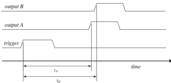
Figure 1: Signals of a delay generator.
