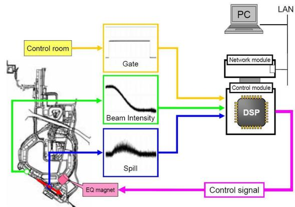
Figure 1: Flow of the signal of the feedback system of slow extraction
