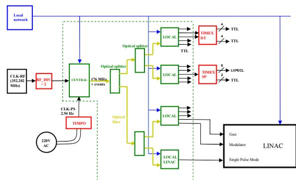
Figure 1: SOLEIL synchronization system architecture.
