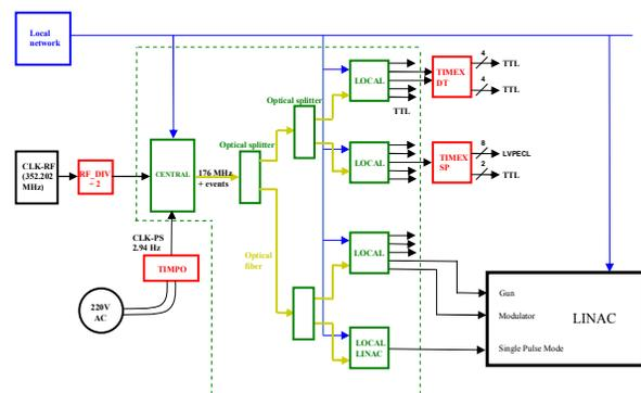
Figure 1: SOLEIL synchronization system architecture.
