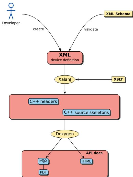
Figure 2: Workflow for the generation of C++ sources and API docs from XML device definition.
