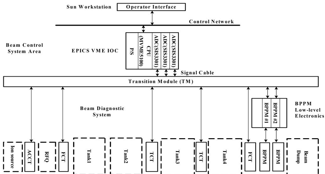
Figure 1: Schematic diagram of the beam diagnostic and monitoring system.
