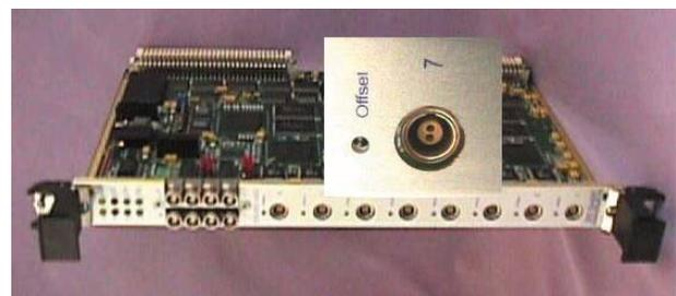
Figure 3: Picture of fast ADC (SIS3301).
