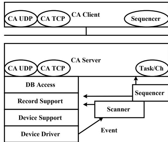
Figure 2: Block diagram of IOC software.
