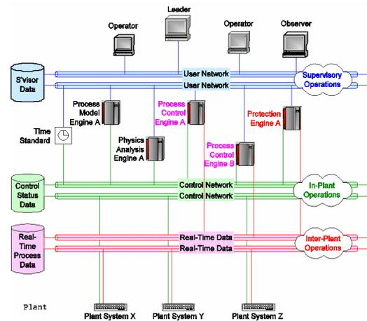
Figure 4: Configurable, Extensible Real-Time Data Network.
