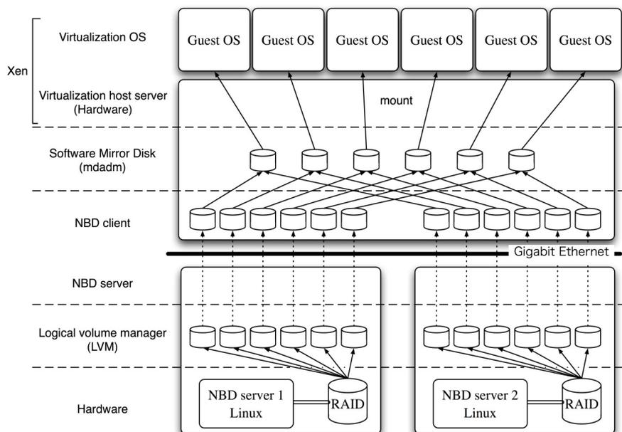
Figure 3: Layout of the Root file system with high availability and high performance.
