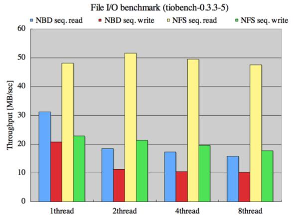
Figure 2 Result of file I/O benchmark program comparison between NFS and NBD. NBD keeps high throughput during multiple access.
