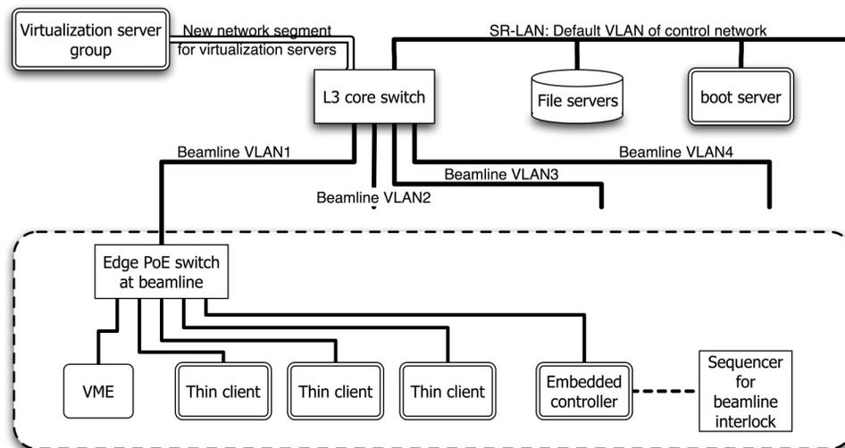
Figure 1 Schematic view of network system for virtualization environment. Components denoted by a double line were newly installed.
